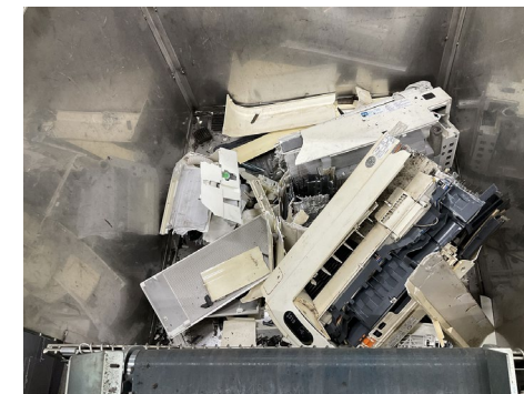
Indoor unit after cutting
